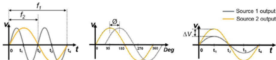
Figure 3. Synchronizing frequency, phase and voltage sources
